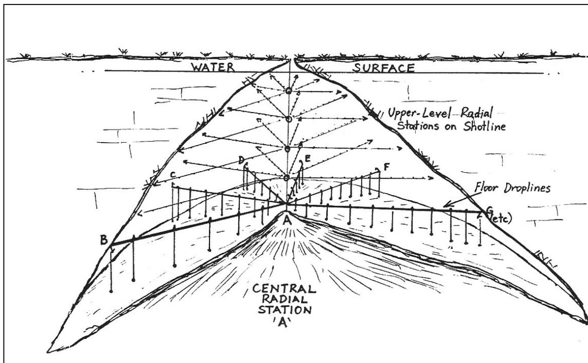
A multi-level (open) **RADIAL SURVEY** from a single (central) reference station; the technique used in mapping "The Shaft" (5L158) by the CDAARG (1983)
