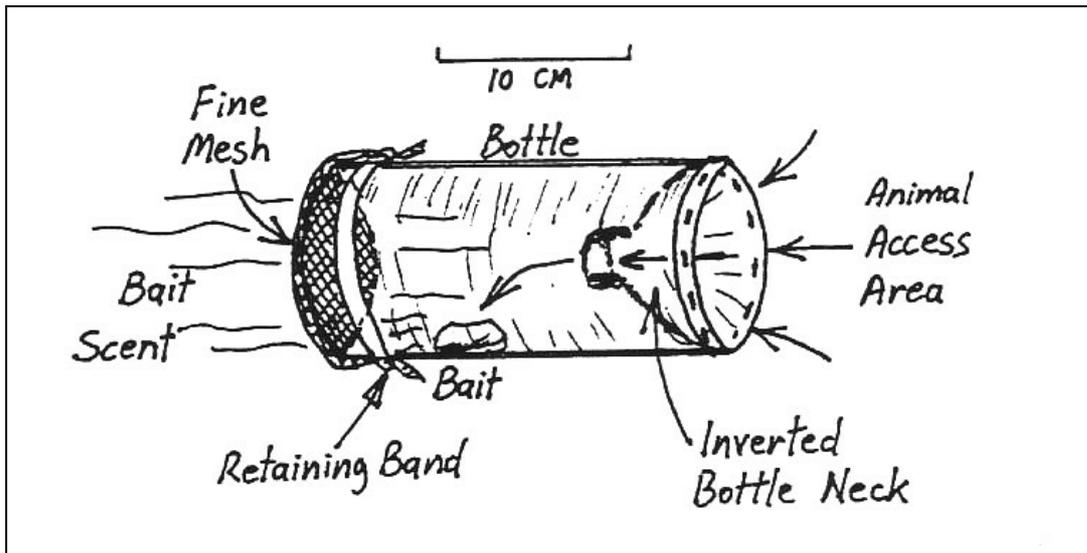
A Basic Inverted-Cone Mesh Trap
