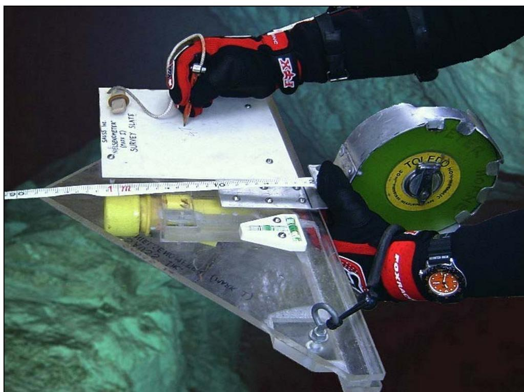
The "Nielsenometer", a combined survey instrument for surveying large waterfilled features (photo courtesy Emi Okada)
